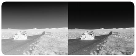
"ACE" - Active Contrast Enhancement™ to dynamically adjust contrast for relative scene temperature
