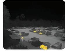
Manually set isotherm thresholds to colorize temperatures of interest (mid-range) in the grey scale
